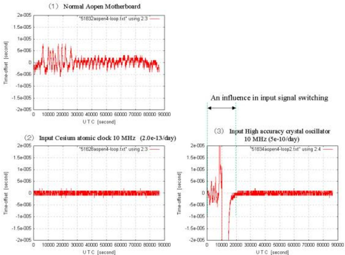
**Figure 2: Time comparison between NTP server and GPS time**
